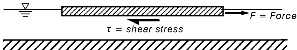
Figure 1.1 Use of a floating board to apply shear stress to a reservoir surface.
